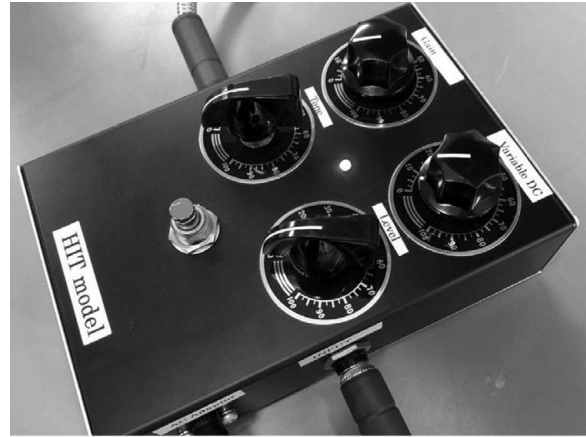
Fig. 5. The newly fabricated distortion pedal has 4 knobs: “Gain,” “Tone,” “Level,” and a “Variable DC” knob that controls the feedback resistance VR4. The variation in distortion is controlled by a combination of the “Gain” knob D1 and “Variable DC” knob D2.
