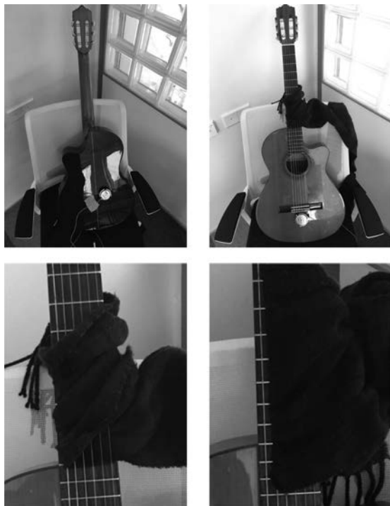
Fig. 2. Experimental setup of the actuated guitar. Positioning of back plate actuator (top left). Muted string configuration for open loop response measurement (top right and bottom left). Open E2 configuration for open loop response measurement (bottom right). The front plate actuator was not used in this work.
