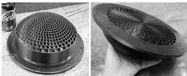
Fig. 3. 3D printed acoustic lens.
