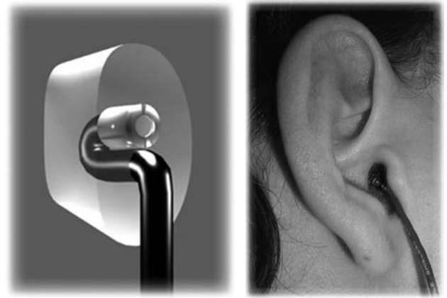
Fig. 1. Custom-built silicone earplug. Left: CAD model, right: inserted into a subject's ear (from [18]).
