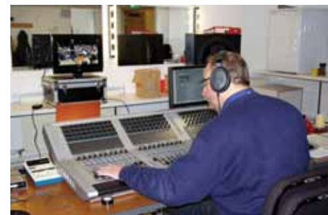
The 32-fader Studer Vista 5 installed at U.K.-based Chandos Records
