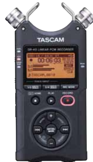
TASCAM's DR-40 4-track portable recorder
