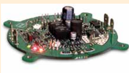
D-fend is an all-digital, programmable loudspeaker protection and attenuation circuit
