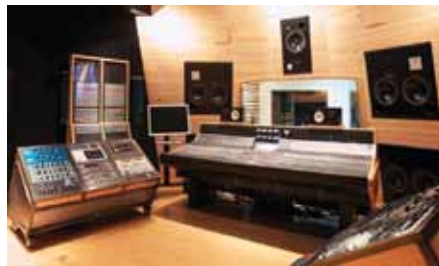
The newly opened 25th Street Recording in Oakland, CA, features an API Vision analog console
